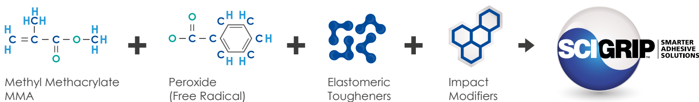
Figure 1: Scigrip MMA adhesives are formed by a free radical polymerisation mechanism which is highly exothermic
